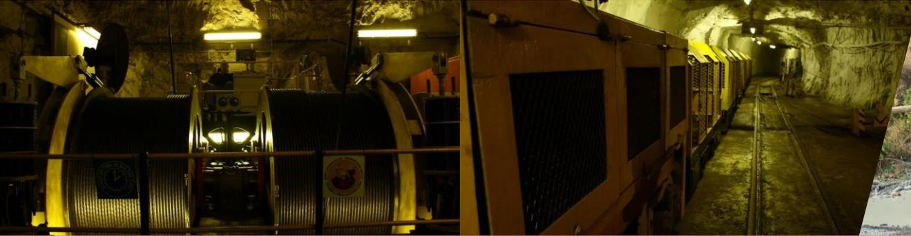
Underground was shaft and rail constrained to 15,000 tonnes per month
