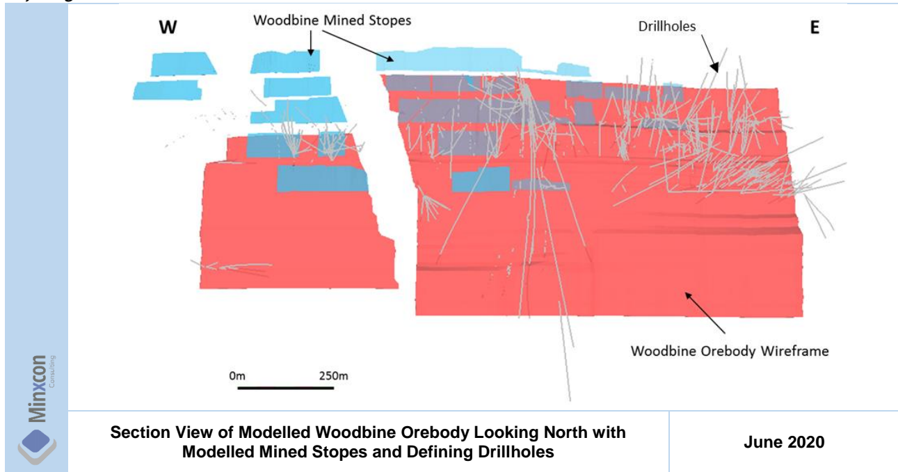
Figure 20: Section View of Modelled Woodbine Orebody Looking North with Modelled Mined Stopes and Defining Drillholes
